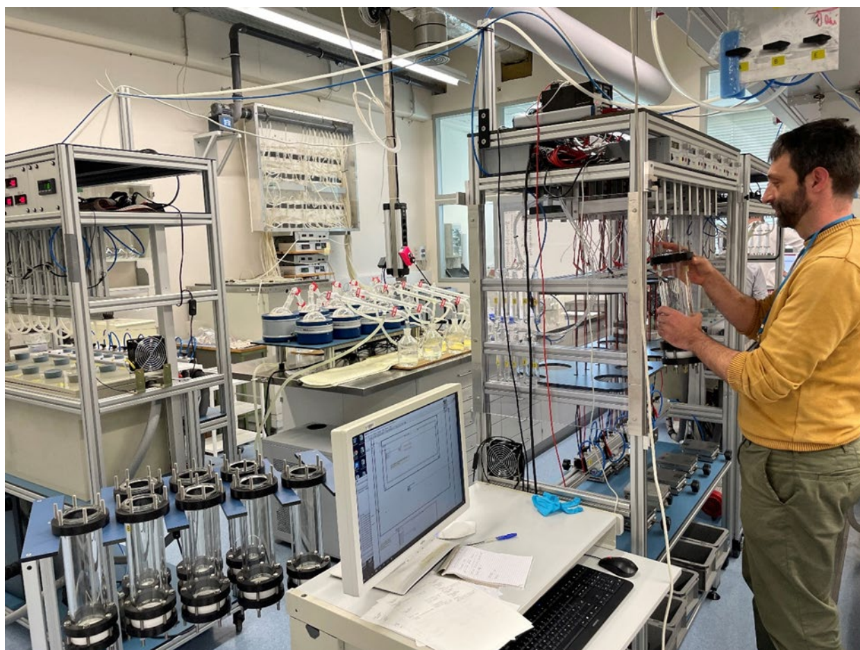
FIG. B.1. New method for tritium enrichment based on solid polymer electrolyte membrane (PEM) technology, with distillation system in background. (Source: IAEA)
