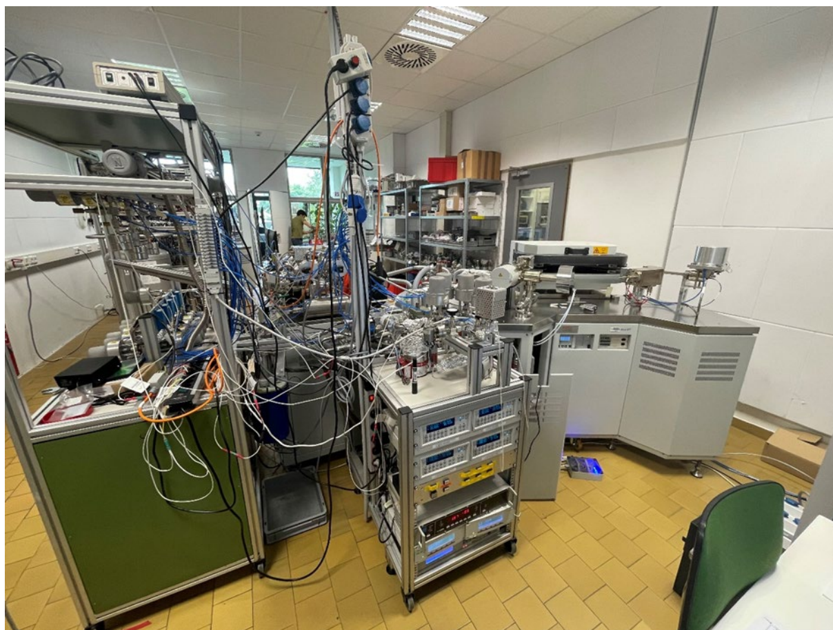
FIG. B.2. The new state-of-the-art helium-3 mass spectrometer system for the analysis of tritium concentrations using the helium-3 ingrowth method installed in the Isotope Hydrology Laboratory. (Source: IAEA)
