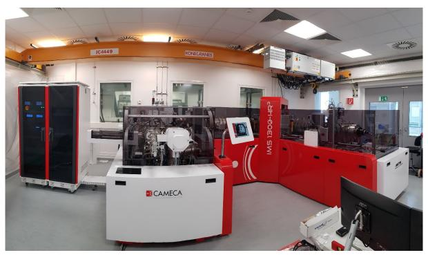
The new Large Geometry Secondary Ion Mass Spectrometer (LG-SIMS) (Photo credit: IAEA staff)
