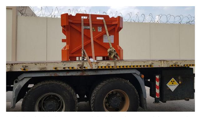
The disused sealed radioactive source packed in the licensed container ready for international transport. (Photo: IAEA Contractor)
