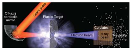
FIG. C-4. Schematic representation electrons and secondary neutrons being produced using laser based accelerating technologies. (Photo: Ishay Pomerantz, Tel Aviv University, Israel)
