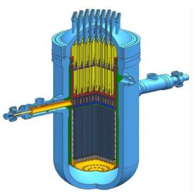
FIG. B-2. Reactor core concept of the Chinese SCWR design. (Source: IAEA)
