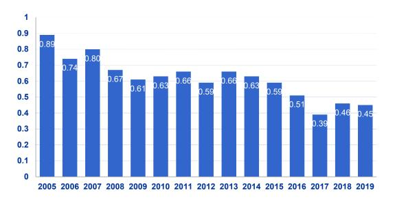
FIG. A-4. Mean rate of scrams: the number of automatic and manual unplanned scrams per 7000 hours of operation of a unit. (Source: IAEA Power Reactor Information System <u>www.iaea.org/pris</u>)
