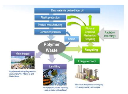
FIG D-1: Life cycle of plastic products and the generation and treatment of plastic waste. (Source: IAEA)
