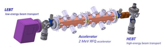
FIG. C-2. Schematic drawing of the main components of MACHINA. The ion beam can be extracted on the high-energy side of the accelerator to analyze the artifact. The very first applications are based on the PIXE technique, where X-rays are generated owing to particle-matter interactions. The emitted X-rays are then detected and, after data evaluation, the sample composition is determined. (Photo: MACHINA project)
