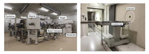
FIG. D-3. Accelerator and target components (left) together with patient irradiation position (right) at an accelerator-based BNCT centre. (Photos: Kansai BNCT Medical Center, Japan).
