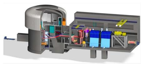
FIG. B-1. Canadian SCWR design: reactor buildings and the turbine building. (Source: IAEA)
