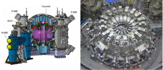
FIG. B-8. Schematic representation of the JT-60SA (left) with a photo of the close-to-completion torus assembly. (Source: P. Barabaschi et al., presented at the 2018 IAEA Fusion Energy Conference)
