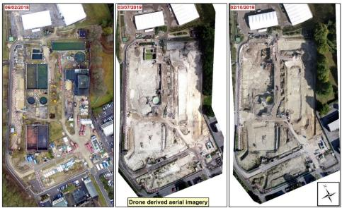
FIG. A-13. Drone-derived aerial imagery showing the progress of remediation of the Liquid Effluent Treatment Plant at the Harwell site, United Kingdom. (Photos: Magnox Ltd)
