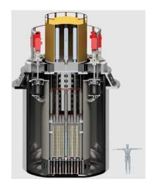
FIG. B-5. 55 MW(e) SEALER-UK LFR design.
