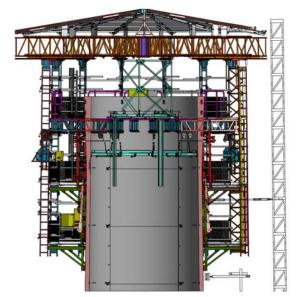
Fig. A-11. Self-climbing platform designed to assist in the demolition of the ventilation stack of a legacy reprocessing plant at the Sellafield site. (Photo: Sellafield Ltd)
