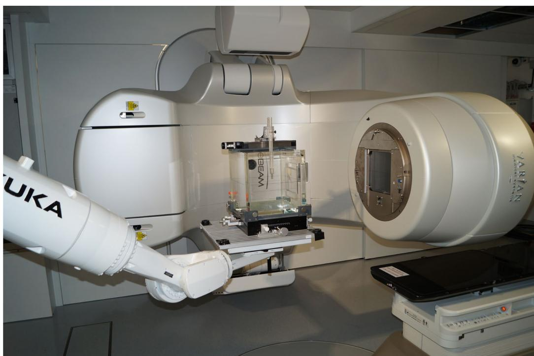
*FIG.B.5 Performing LINAC calibration using the robotic bench at the IAEA Dosimetry Laboratory in Seibersdorf. (Source: IAEA)*
