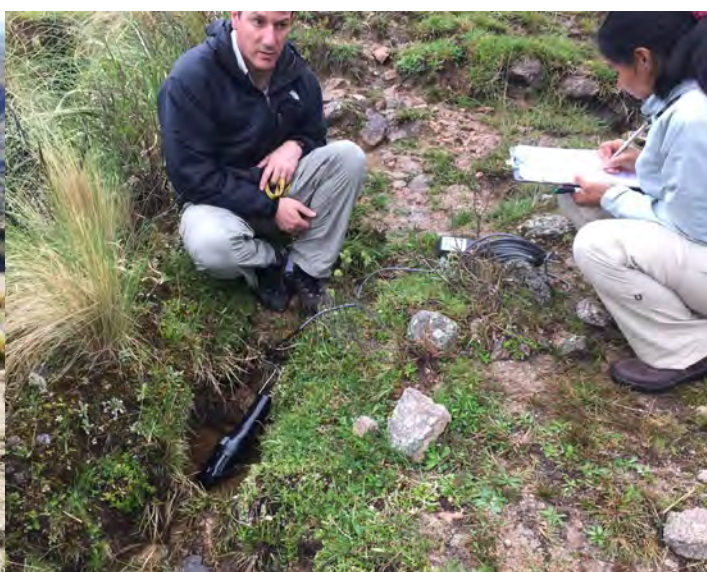
Los Gigantes, Córdoba, Argentina. Measurement of hydrochemical parameters with a multiparametric sonde. Photo: CNEA, Argentina.
