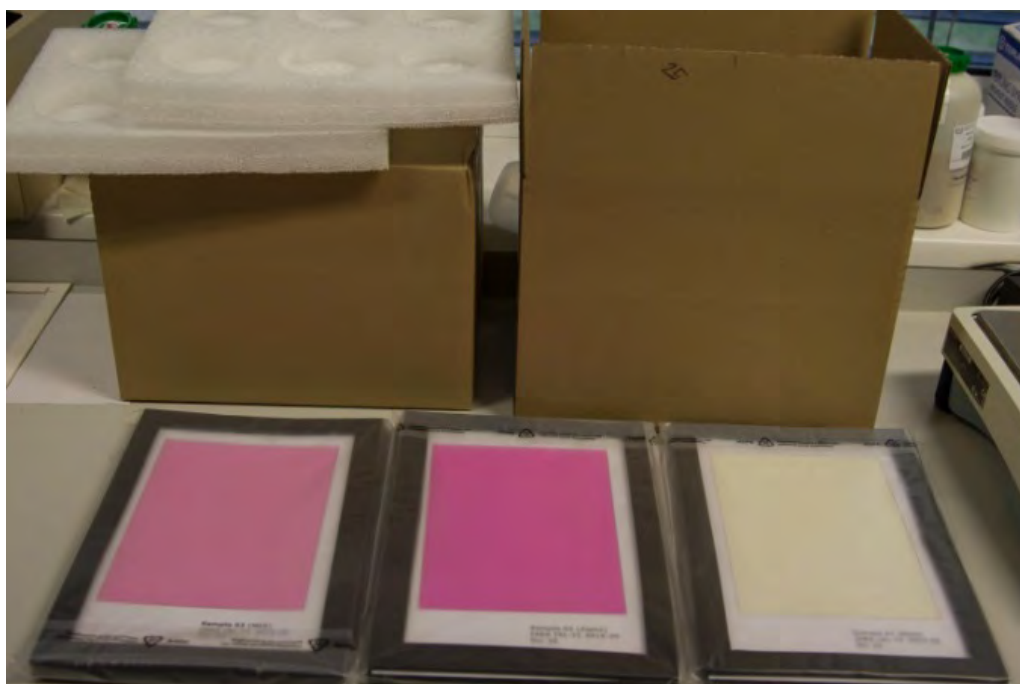
RER7008: Proficiency test under RER7008: Shipment of novel reference materials with radionuclides imprinted homogeneously by ink printers on paper sheets (each color denoting a different radionuclide). Photo: S. Tarjan/IAEA.
