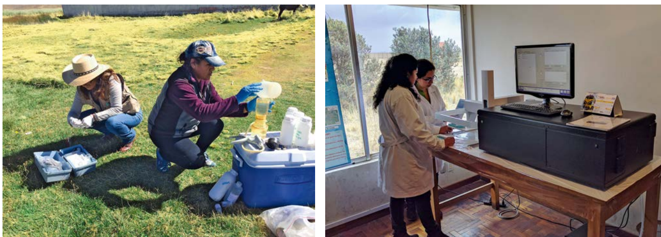
FIG. 1. As part of a technical cooperation project, Bolivian counterparts collect groundwater samples in the field (left), which are then analysed to measure the isotope ratios using a laser analyser provided by the Agency (right).
