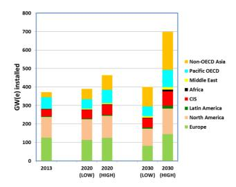
FIG. 3. Regional capacity developments in the low and high projections. Source: Based on IAEA-RDS-1, 2014 Edition.
