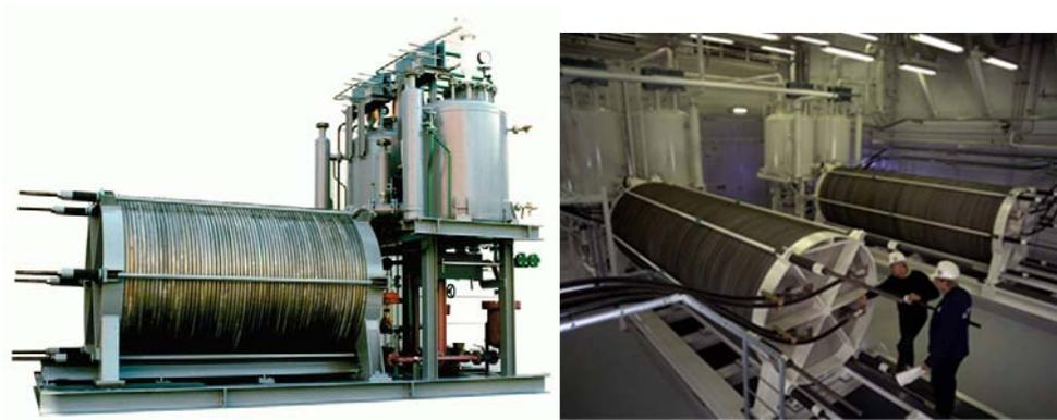
*FIG. 1. Standard low temperature alkaline electrolysis.*
