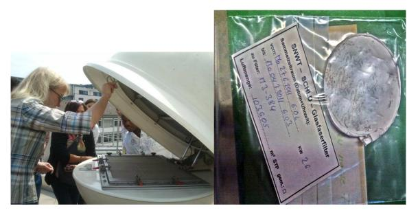
FIG. F.1. Large volume aerosol collector operated by the Federal Office for Radiation Protection in Salzgitter, Germany, and aerosol filter compacted for immediate gamma spectrometric counting being demonstrated to participants in the Agency's Interregional Advanced Training Course on Marine Radioactivity: Analytical Techniques and Quality Management hosted by the Karlsruhe Institute of Technology in 2011.
