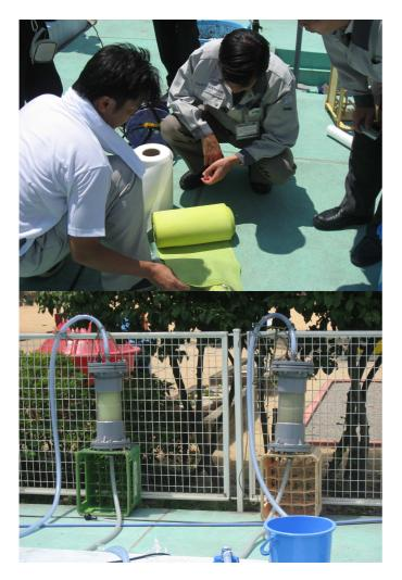
FIG. H.1. Grafted membranes being used for removing radiocaesium from water in the Fukushima area (courtesy of JAEA Takasaki, Japan).
