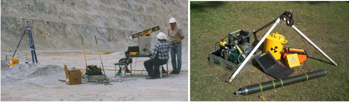
*FIG. III-6. PGNAA borehole logging for copper grade analysis in Chile.*
