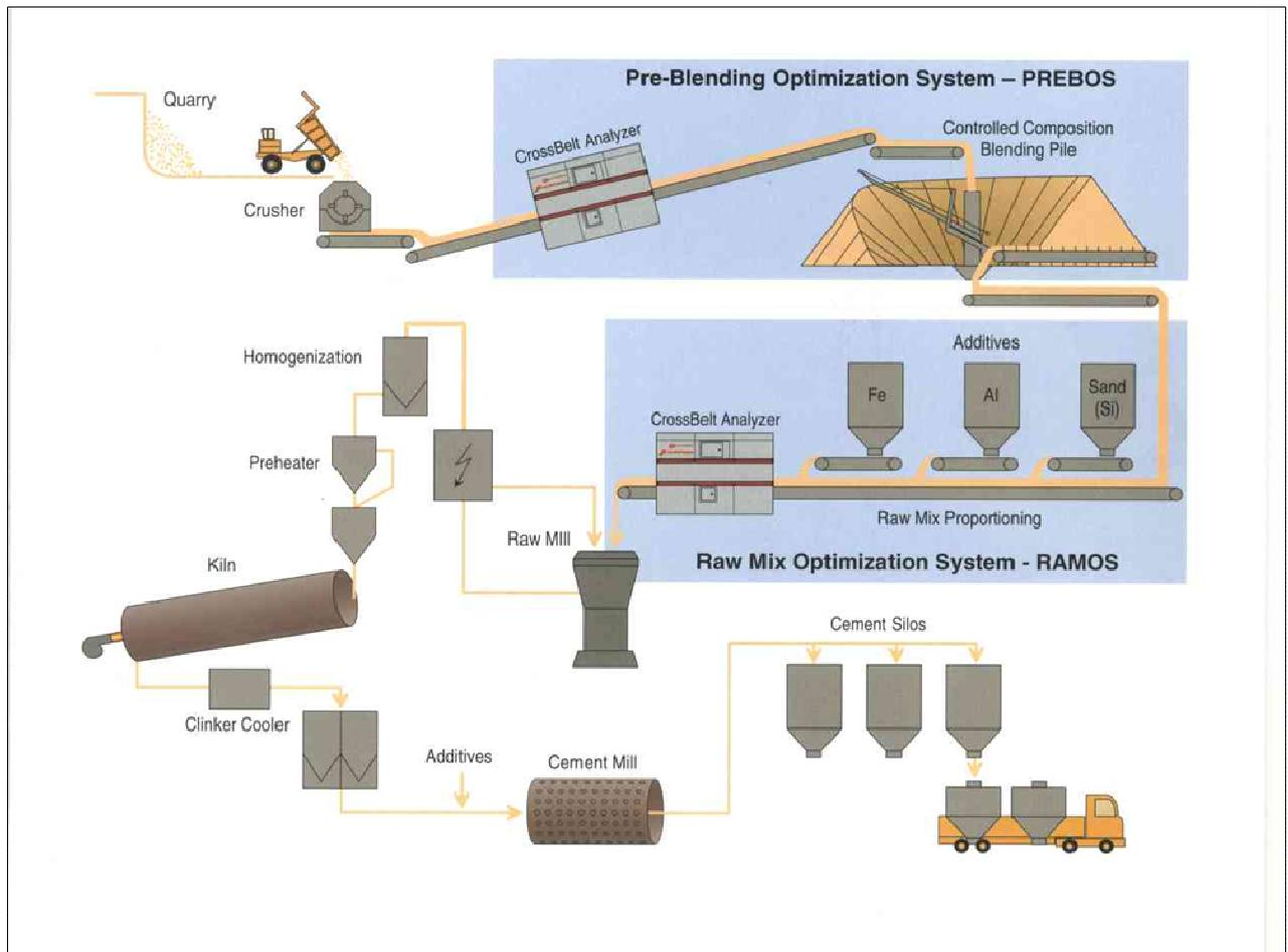
FIG. III-7. The schematic design of PGNAA equipment in a cement plant in Thailand.
