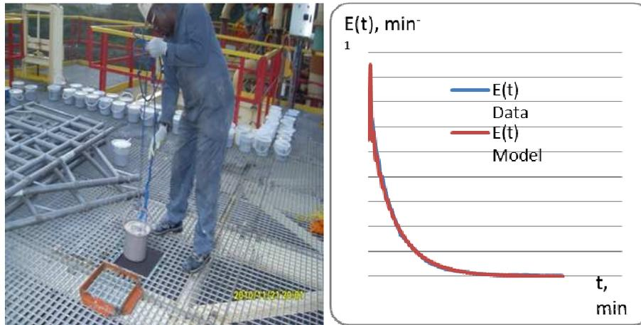
FIG. III-2. Experimental RTD sampling and modelling.
