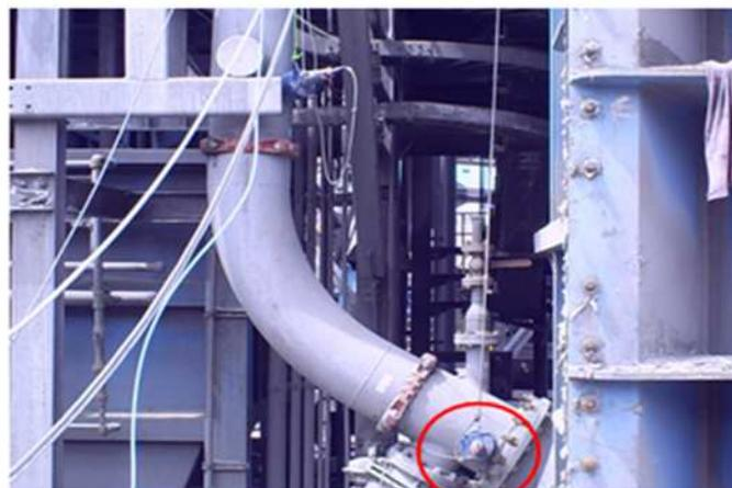
FIG. III-3. Experimental RTD measuring point.
