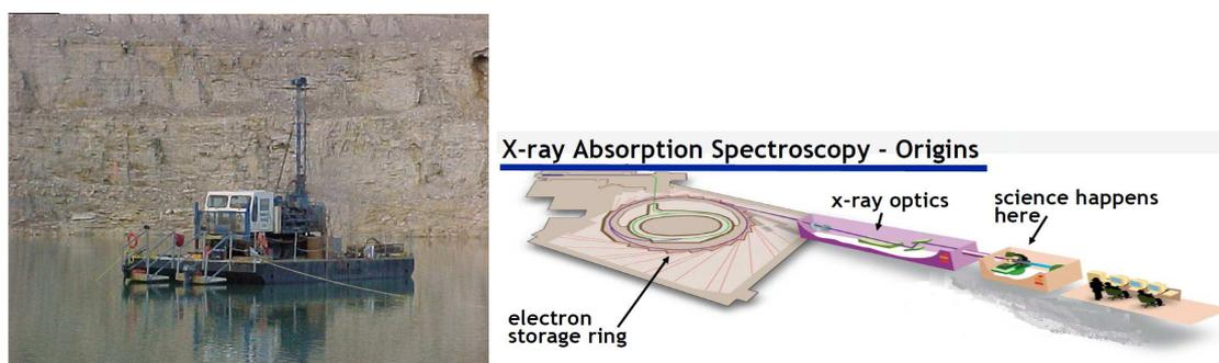
*FIG. III-8. Left: A barge mounted drill rig at the mine site was used to sample pore waters and to obtain cores of the tailing material. Right: X-ray absorption experiment schematic design at the synchrotron facility.*
