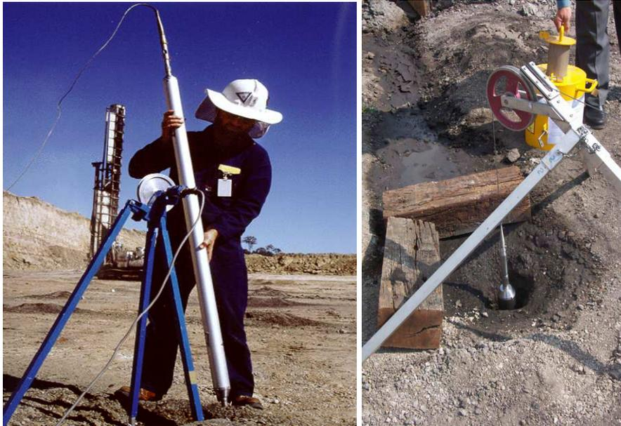
*FIG. III-5. Low radiation intensity (1.1 MBq) gamma spectrometric borehole logging probe for coal delineation and coal raw ash content.*
