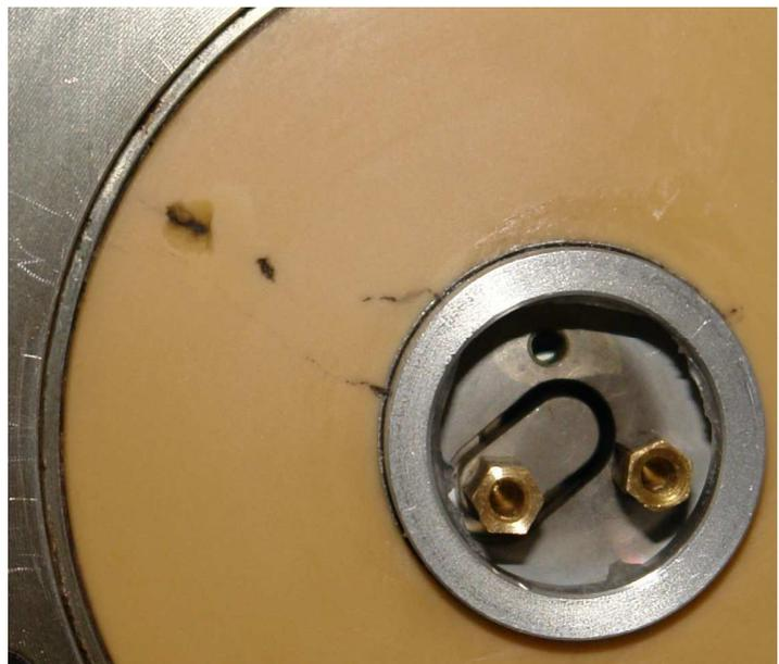
*FIG. I-2. Detail of X-ray tube end cap insulator showing damage caused by high voltage arcing.*
