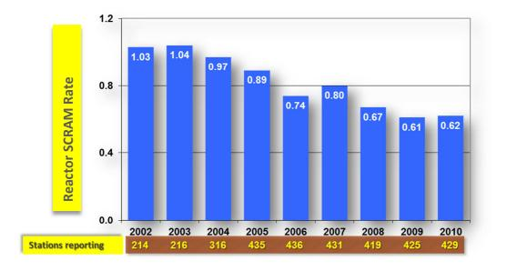
FIG. 1. Total number of unplanned reactor shutdowns ('scrams'), including both automatic and manual scrams, which occurred per 7 000 hours of critical power reactor operation.
