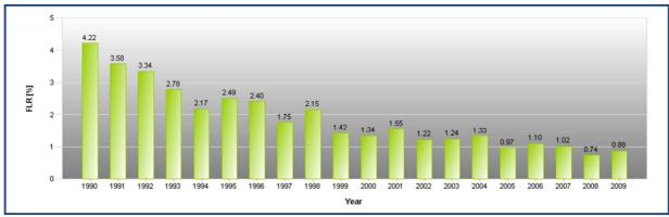
Figure 2: Forced loss rate data (source: 2010 Performance Indicators, World Association of Nuclear Operators)
