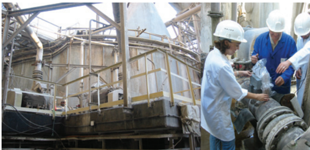
FIG. 3. Optimizing phosphoric acid production using radiotracer techniques at a plant in Tunisia.
