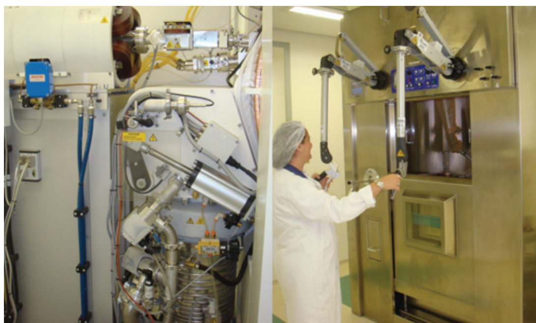
FIG. 2. A cyclotron beam extractor (left) and production hot cell (right) for manufacturing PET radionuclides in Recife, Brazil.
