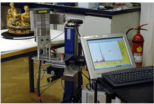
The IAEA has developed a mobile XRF spectrometer, which can easily be carried into museums or archives for in situ measurements
