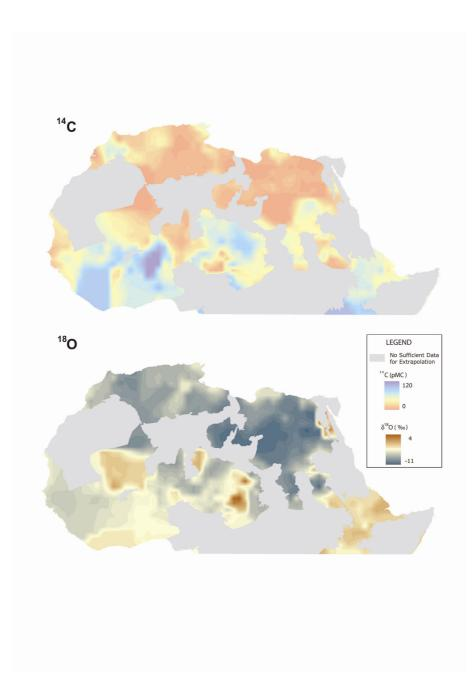
FIG. H-1. Carbon-14 and oxygen-18 contents in groundwater in northern Africa from the recently published IAEA Atlas of Isotope Hydrology. The low carbon-14 values show the extent of 'very old' groundwater that was recharged under wetter climates thousands of years ago.
