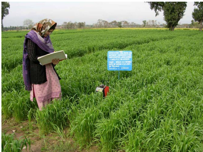
PIC. 2. Better irrigation management by using a soil moisture neutron probe.
