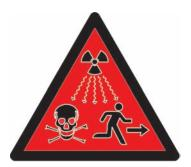
FIG. 3. The new radiation warning symbol to supplement the existing trefoil sign.
