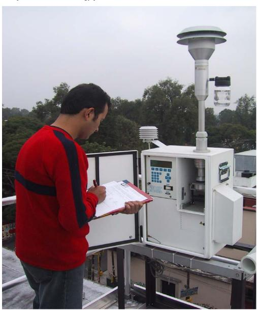
FIG. 11. A technician collects current operational data from the fine particle air sampler at the atmospheric sampling site at Coyoacán, in the greater metropolitan area of Mexico City. (Photo courtesy of the National Nuclear Research Institute, Mexico.)
