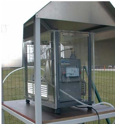
Fig. H-3: A high volume air sampler, for use in air pollution or radon monitoring
