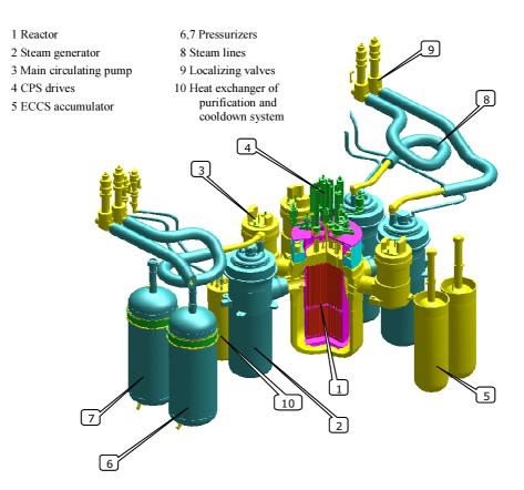
FIG. 2. Modular layout of the KLT-40S reactor plant (Source: OKBM, Russian Federation).
