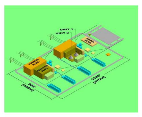
FIG. 4. Perspective view of IRIS multiple twin-unit site layout (Source: Westinghouse, USA)
