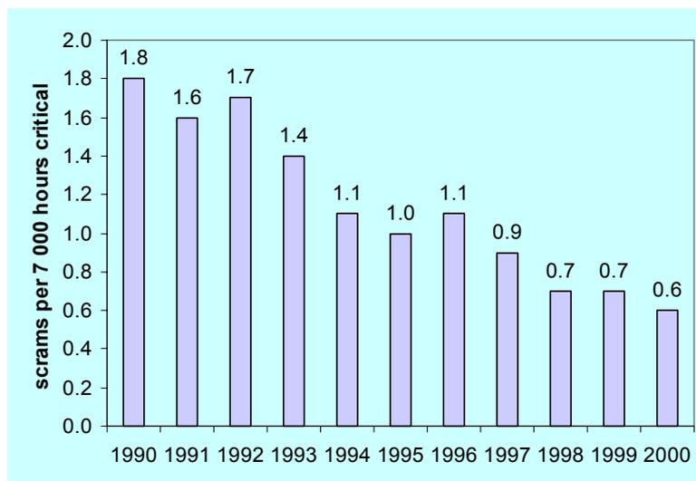
Figure II-1. Unplanned automatic scrams per 7 000 hours critical
