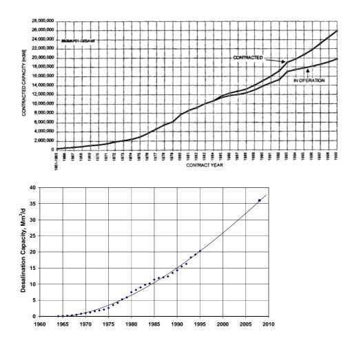
Fig. 2. Cumulative worldwide desalination capacity. The top line in the top figure shows total operating and contracted capacity. The bottom line in the top figure shows just operating capacity. The bottom figure shows projected growth including both operating and contracted capacity. Data source for all historical data: Wangnick, 2000; informal projection based on IAEA Consultancy Meeting.
