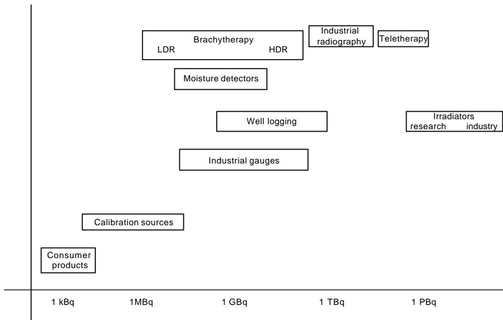
Figure 1. Activity ranges for some important applications of sealed sources
