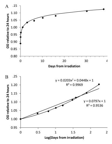
Figure 12. Change in OD of Gafchromic<sup>TM</sup> HD-V2 film with time. A: linear time up to 38 days; B: Log time to 174 days
