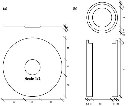
Figure 17. Typical support design (stand) for dosimeter holder for use in a Gammacell. Recommended material is PMMA. All dimensions are in mm.
