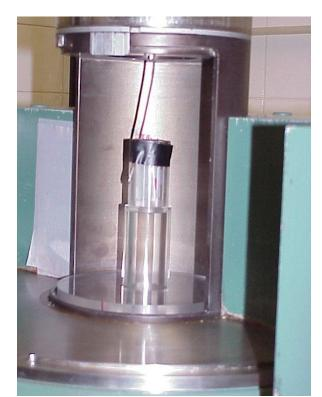
Figure 23. Three dosimeters in a cylindrical dosimeter holder on a stand are prepared for irradiation in a Gammacell. Thermocouples are used to measure the temperature throughout the irradiation, where the thermocouple junction is located inside the dosimeter holder next to the dosimeters. A black tape is used to hold the wires firm in position. The wires leave the irradiation chamber through the central access tube to the recording device situated outside the Gammacell.
