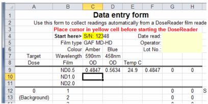
Figure 10. Data entry form with the headers and the first ND filter reading. The DR4 should be started as above and the cursor placed in the bright vellow cell (C4).
