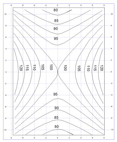
Figure 14. Typical dose-rate distribution in the irradiation chamber of a Nordion Gammacell-220. The values are normalised to 100 in the centre of the gamma field. Note that the field is most uniform in the centre. (Grid is at 2 cm intervals from the centre of the chamber). Re-drawn from Nordion data.
