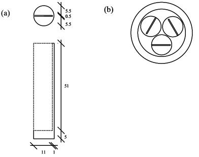
Figure 22. (a) Gafchromic<sup>TM</sup> film holder and (b) the arrangement of three such holders in the cylindrical dosimeter holder. Note that all the three films are parallel (tangential) to the curved surface of the dosimeter holder. All dimensions are in mm.
