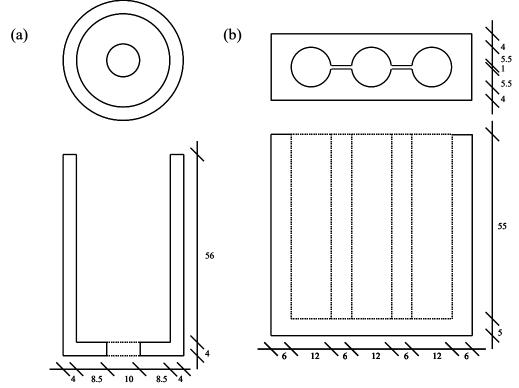
Figure 15. Two dosimeter holder designs for use with different types of irradiators. Recommended material is PMMA. (a) for self-contained irradiators, note hole in the bottom that facilitates natural air circulation; (b) for panoramic irradiators. All dimensions are in mm.
