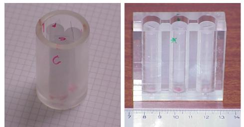
Figure 16. Two types of dosimeter holders to accommodate three dosimeters for simultaneous irradiation: (a) this cylindrical (open cup) type is suitable for irradiation in self-contained irradiators like Gammacell and Husman-type, where the gamma source surrounds the dosimeters and the field is isotropic, and (b) this flat holder is suitable for panoramic irradiators which have a plane or a rod source and the gamma field is unidirectional. These holders are made of PMMA.
