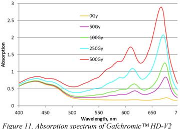
Figure 11. Absorption spectrum of Gafchromic<sup>TM</sup> HD-V2 film at various doses.
