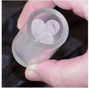
Figure 21. Three film holders with  $Gafchromic^{TM}$  dosimeters are placed in a cylindrical dosimeter holder for irradiation in a Gammacell. Note that each film holder is placed so that the film is parallel (tangential) to the curved surface of the dosimeter holder. For a flat dosimeter holder, the film holders should be placed so that the films are parallel to the longer face of the dosimeter holder.
