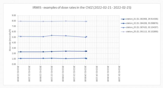
Fig. 1: Single dose rate measurements at four locations within the Chornobyl Exclusion Zone received by IRMIS before 24 February. Despite events within this area, radiation measurements taken by staff at the Chornobyl NPP site indicated that rates remined low and did not pose any radiological hazard.
