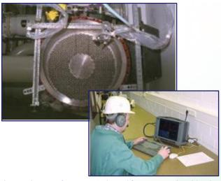
Inspecting non-ferromagnetic and ferromagnetic tubing in petrochemical, chemical and power generation plants.
