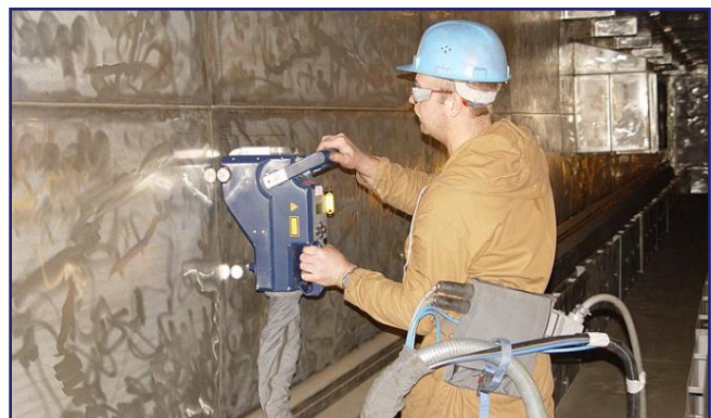
Demonstrating a hand laser, Workshop on Cutting Technologies for Decommissioning, Germany, 2011.
