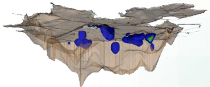
*Three dimensional model grid for the NSAS showing the effects of pumping.*
