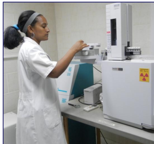
CEAC staff operating a gas chromatograph coupled with mass spectrometer to survey petroleum hydrocarbons in marine samples.
