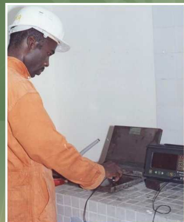
Carrying out ultrasonic testing of a weld.
