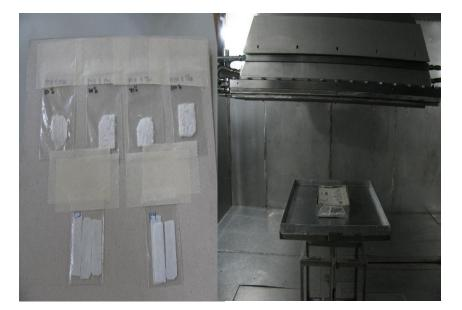
Strips of abaca and polypropylene nonwoven fabric for irradiation Irradiation position of abaca and polypropylene nonwoven fabric
