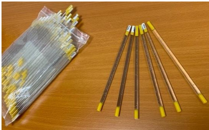
Figure 3: Rod sources used in the ALPS interlaboratory comparison on in vivo radiobioassay.
