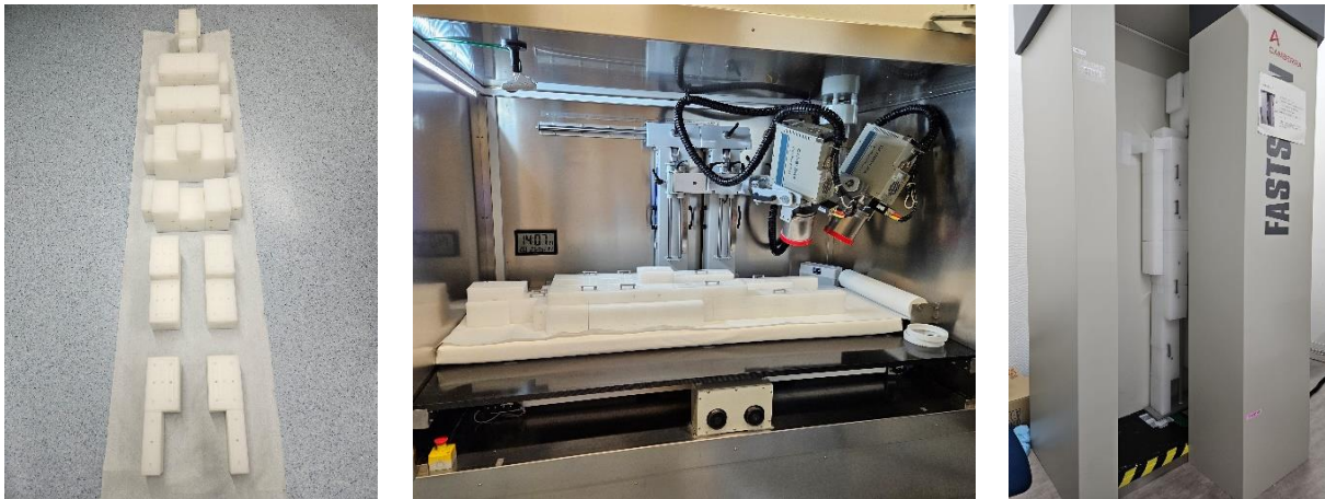
Figure 2. The F4-size UP-02T unified brick phantom consisting of rectangular polyethylene bricks set up in a stretcher and standing geometry.
