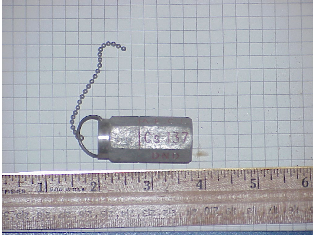
Figure J.1: Cesium-137 radioactive sealed source
