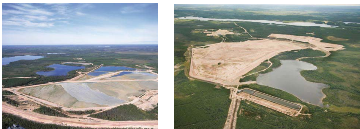
Figures 7.3 (a) and (b) – Photographs show the Cluff Lake TMA during operation and after decommissioning but prior to the revegetation becoming established.
