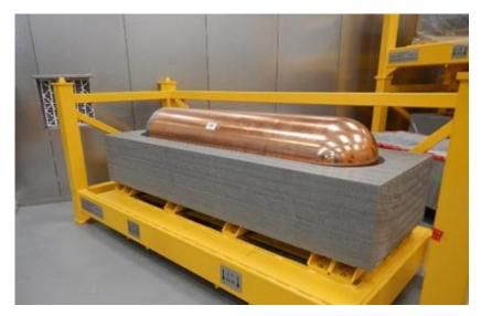
The NWMO is also developing non-destructive examination techniques and custom equipment to inspect the UFCs following the various stages of fabrication, such as welding, copper coating and machining. These inspections will ensure that UFCs meet the required specifications.
