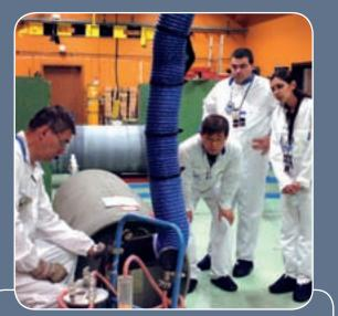
Another step for inspectors is to verify levels of enrichment during the uranium conversion process. Here inspectors observe a plant operator carefully extracting a UF6 sample to be analyzed for isotopic composition.
