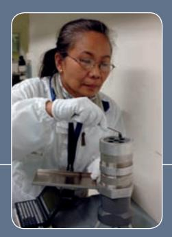
An inspector verifies the pellet's enrichment using an instrument called a Mini-Multichannel Analyzer that attaches to a palm-sized computer.
