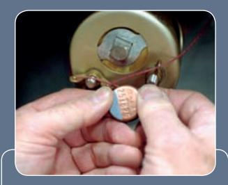
Once the cylinder's contents are verified, inspectors attach an IAEA metallic seal — commonly used to prevent tampering. The seals provide important evidence of any unauthorized attempt to gain access to the secured material.
