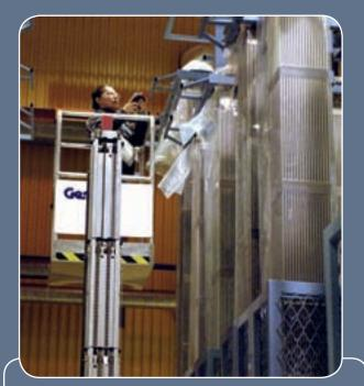
Going up to the source is sometimes the only way to access the assemblies for critical measurements. In this case, an inspector is hoisted into the air on a crane to get an active length measurement.
