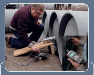
Checking the cylinder is one thing. Checking what's inside is another. Inspectors rely on sophisticated instruments — such as germanium detectors and sodium iodide, pictured here, to detect enrichment levels — most enriched material emits gamma rays. These tools of the trade help inspectors verify the accuracy of the facilities' records.
