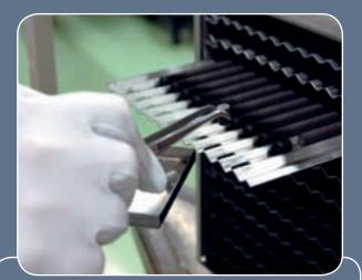
Metal boxes hold trays of finished fuel pellets. Each pellet, slightly larger then a pencil eraser, contains enriched uranium dioxide that will be used at nuclear power plants.
