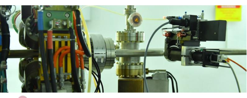
These are sealed vacuum pipes through which the electromagnetic beams pass to reach the experimental hubs.
