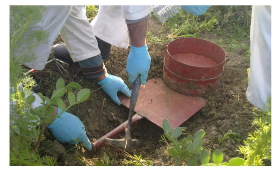
Scientists taking a soil sample during the study of erosion hot spots, using nuclear techniques. (Photo: INRA)
