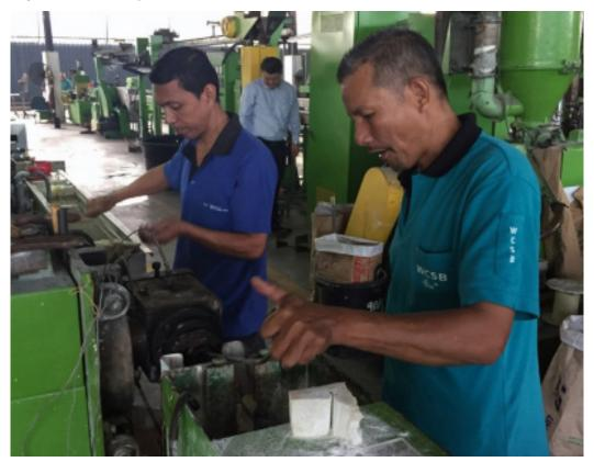
Cables such as these produced at Wonderful Ebeam Cable will be used in the engine compartment of cars. They are made heat resistant and fire retardant using irradiation. (Photo: M. Gaspar/IAEA)
