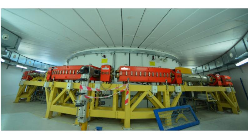
This is the inner storage ring of the facility, where electrons start to circulate to build up the required energy of 2.5 GeV. The inner storage ring, or booster, with deflection and focused magnets, will enable the electron beams to circulate as they accelerate. The precise beams of light produced include microwave, infrared, visible, ultraviolet, X-ray and gamma-ray light.
