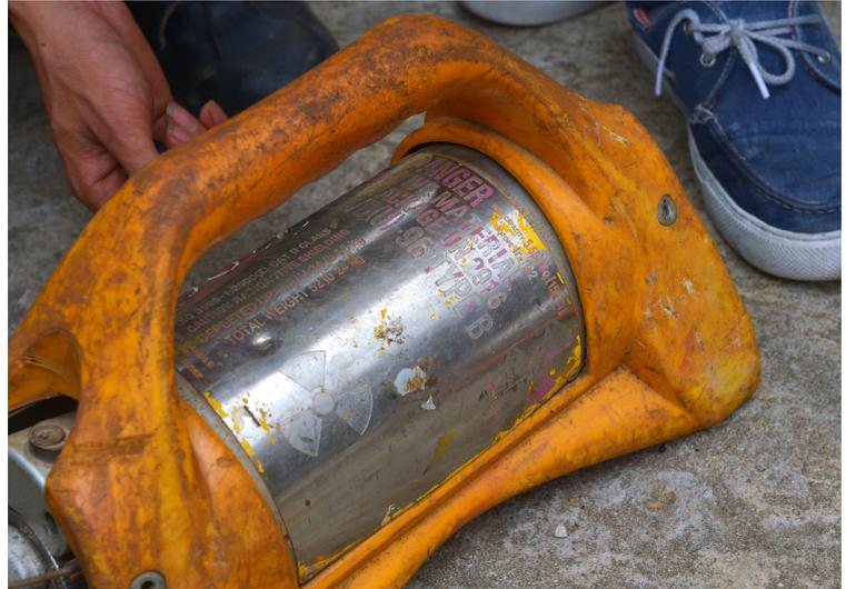
**2** In a similar way that X-rays are used to check for cracks in bones, industrial radiography devices are used to check for cracks or flaws in industrial components. These devices contain radioactive sources and are portable, making them vulnerable to loss or theft. Each year, cases of lost or stolen radioactive sources are reported to the IAEA.
