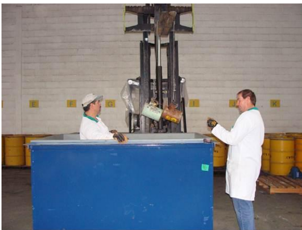
Figures I.1 – (a) B-25 box loaded with disused industrial gauges, (b) transport shields with brachytherapy and industrial sources removed from original gauges
