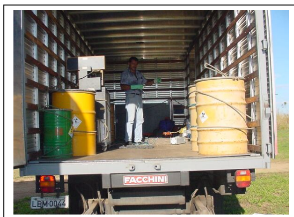
Fig J.2. Type A Waste Containers
