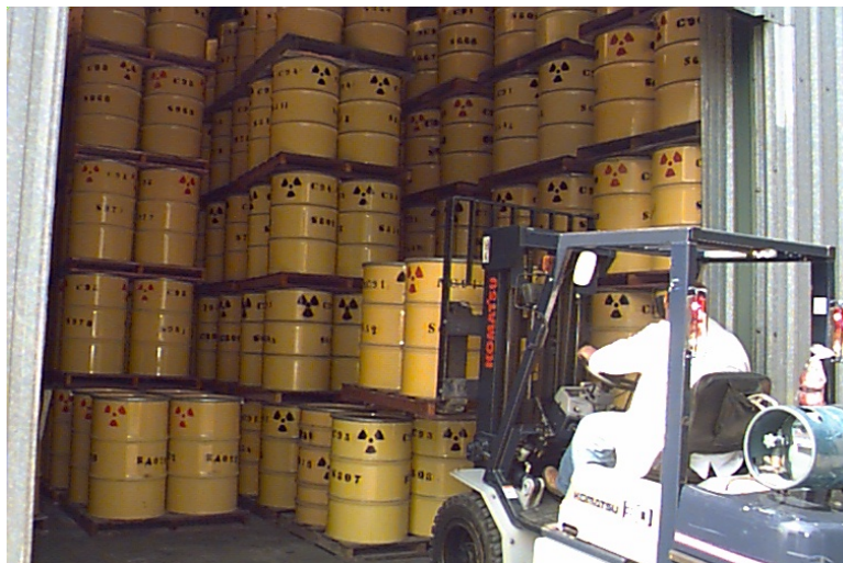
Fig. H.2. Interim Storage of Treated Waste at IPEN
