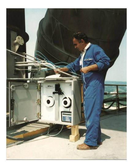
Level gauge - Online measurement of residue liquid butane weight in butane cylinders on LNG bottling carrousels (neutron backscattering - <sup>241</sup>Am-Be)
