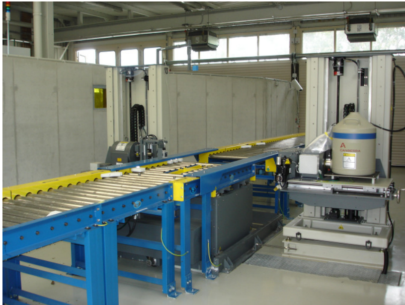
Waste Assay System in the measuring facility at Seibersdorf
