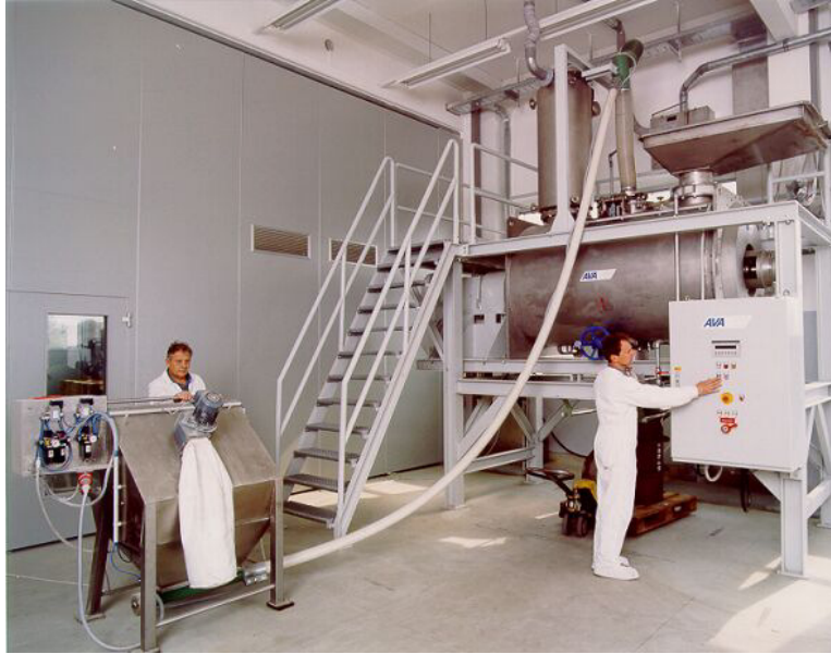
Cementation equipment (used previously)
