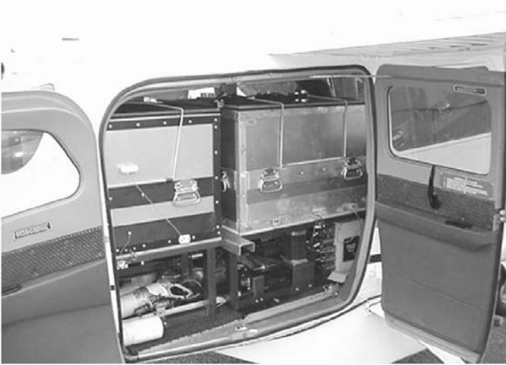
Figure 4. Second generation chilled adult release system installed inside a Cessna 206 aircraft.
