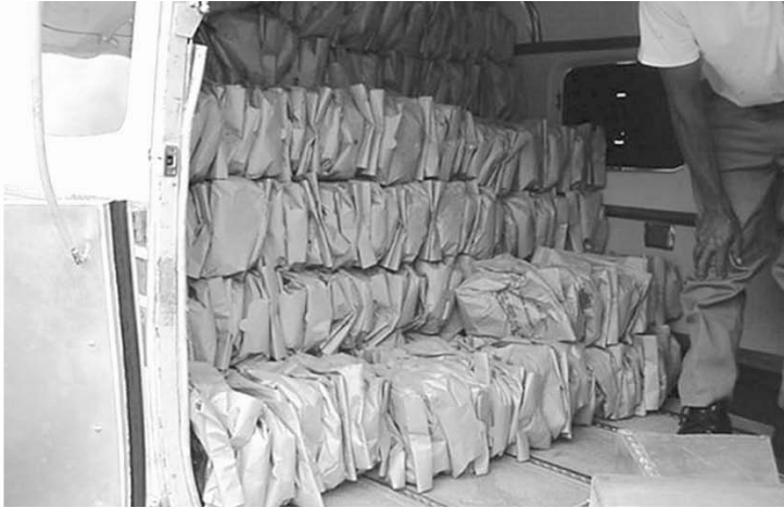
Figure 1. Paper bags stacked in the aircraft cabin prior to release through a chute constitutes the paper bag delivery system.
