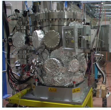
The ultra-high vacuum chamber (UHVC) end station at the IAEA beam line at the Elettra synchrotron in Trieste, Italy. This state-of-the-art X-ray fluorescence beam line can be used to analyse which chemical elements are found in a material. One of the advantages of this advanced technology is its ability to produce 2D and 3D maps showing the chemical analysis of the material being tested. (Photo: IAEA)
