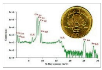
A graph of an ion beam analysis of a Lebanese 250 lira coin to determine its layer composition and thickness. This kind of analysis through nuclear technology can be used to assess and authenticate coins or other ancient artefacts.
