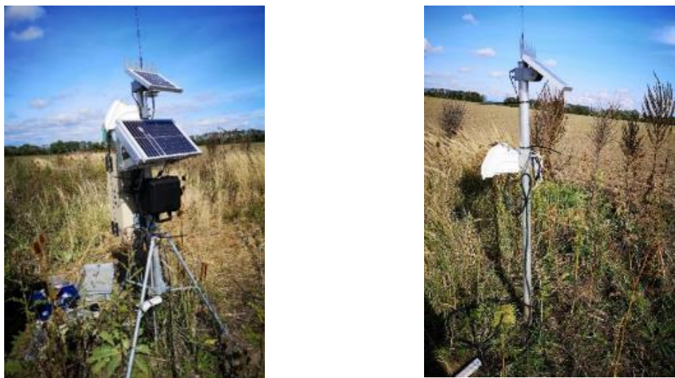
FIG. 4: Cosmic Ray Neutron Sensor (left); one of the capacitance probes (right) installed in Rutzendorf, Austria
