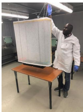
FIG. 10. Blood feeding of 12 000 female Aedes albopictus with a collagen blood sausage in the new mass-rearing cage
