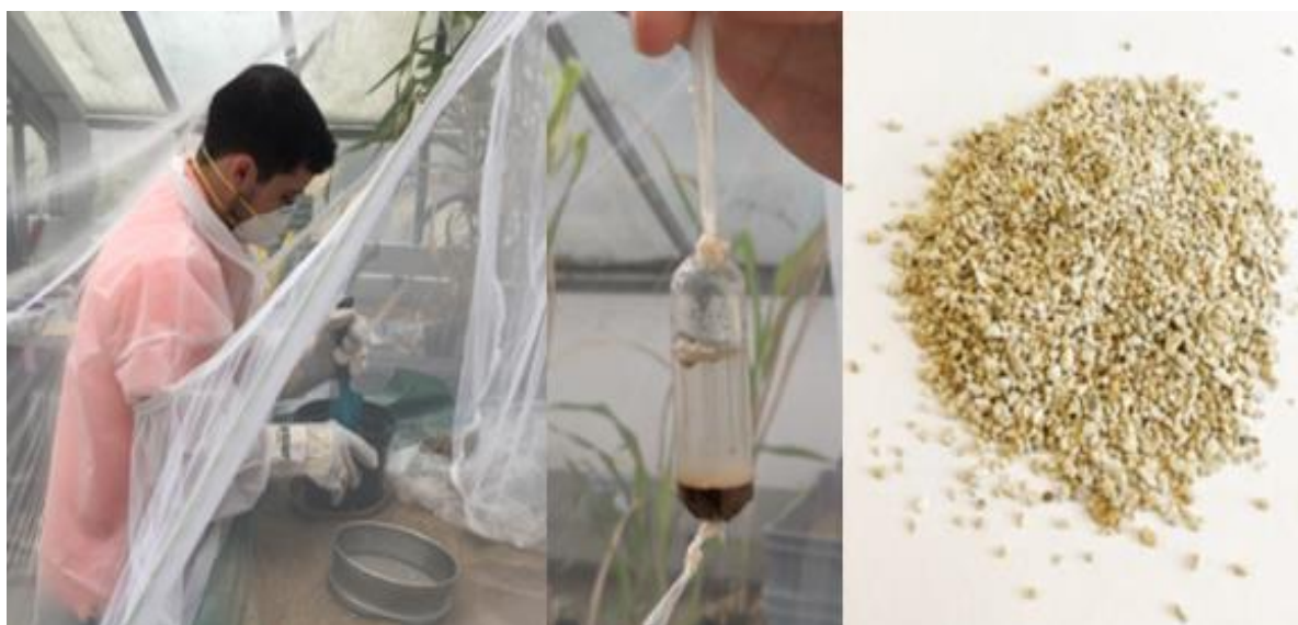
FIG. 8: From left to right: (i) Preparation of soils, (ii) Dialysis bags with soil samples for RIP analysis, (iii) Zeolite minerals.
