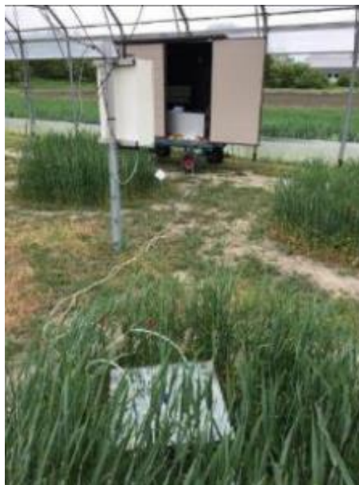
FIG. 2: N_2O measurement on a lysimeter, using off-axis Integrated Cavity Output Spectroscopy (OA-ICOS).
