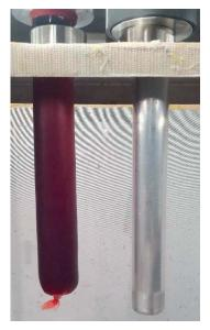
FIG. 11: Sausage heating device developed at the IPCL to reduce the amount of blood necessary to feed a mass-rearing cage.
