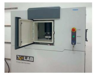
FIG. 6: Nuctech X-Lab prototype twin horizontal beam X-ray irradiator © A.G. Parker
