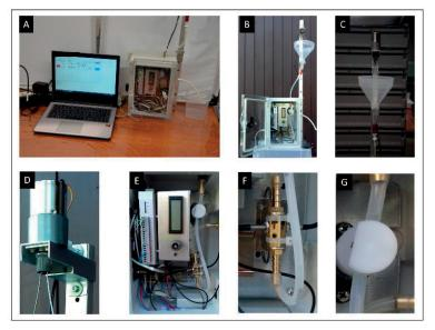
FIG. 9: The automated mosquito larval counter. General view of the larval counter (A); general display of the electronic counting unit and the input larvae container (B); funnel as input larvae container (C); stirrer unit (D); electronic counting unit (E); optical sensor head (F); pinch valve (G).
