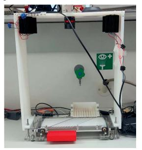
FIG. 5: Prototype of a near infrared spectroscopy system to separate male from female tsetse pupae
