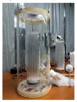
FIG. 12: A prototype flight test device for Anopheles arabiensis
