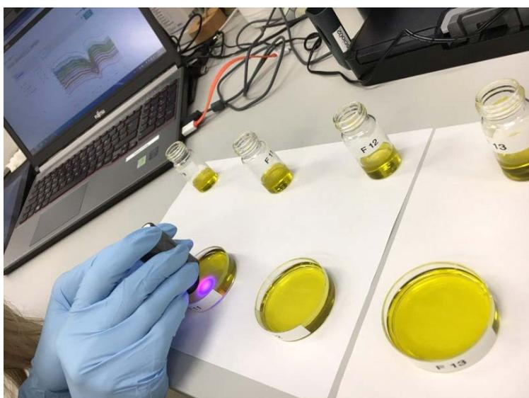
*The hand-held ‘SCIO’ infra-red detector being used to develop a screening test for authentic extra-virgin olive oil*
