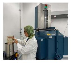
FIG. 4. Ms Arooj Nawaz preparing the male Glossina palpalis gambiensis pupae to be sterilized with the FOSS Model 812 irradiator.
