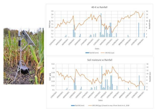
**Figure 2.** Gamma Ray Sensor (GRS) data (<sup>40</sup>K) and derived soil moisture information in relation to rainfall events, in the SWMCNL experimental fields of Rutzendorf (Austria).
